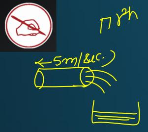
Question 16- Water is flowing at the rate of 5 m/sec through a pipe of diameter 28 cm into a rectangular tank which is 50 cm long, 44 m wide. The time taken for the rise in the level of water in the tank to be 7 cm is
