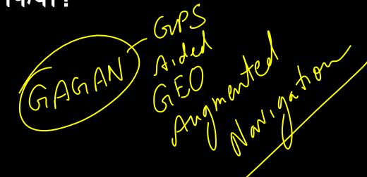
GAGAN (GPS Aided GEO Augmented Navigation) is an Indian satellite-based augmentation system that provides accuracy needed to rely on GPS for flight.
