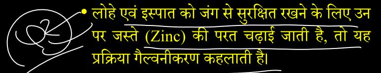
• To keep iron and steel safe from rust, a layer of zinc is applied on them, then this process is called galvanization.
