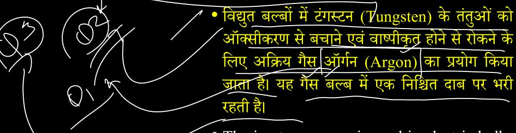
• The inert gas argon is used in electric bulbs to protect tungsten filaments from oxidation and vaporization. This gas is filled in the bulb at a certain pressure.
